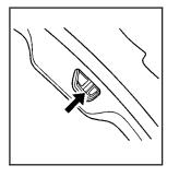
To open the liftgate if the vehicle's battery is disconnected or the voltage is low, access the release lever.
